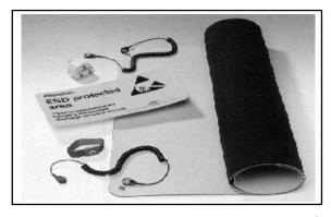
It is recommended that all areas where ESDS devices and assemblies are handled outside their fully protective packaging (assembly, test, inspection, kitting, packaging, etc.), should be provided with a static control work station.
